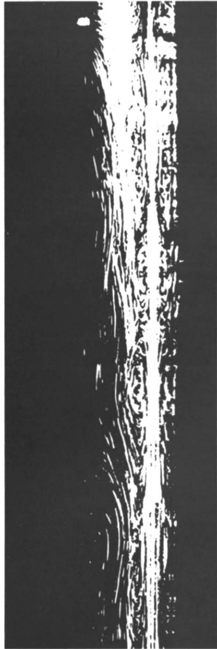
FIG. 5. Steady flow pattern for t_{\infty} = 3.1^{\circ}\text{C} and q'' = 587 \text{ W m}^{-2} in the range 57 < x < 118 \text{ cm} . A strong outer downflow is observed. Inner upflow entrains in the form of discrete vortices.
